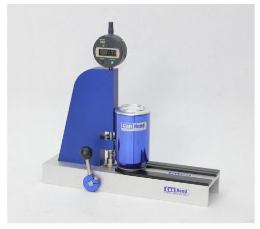
The CanNeed-SLG-d Seam Length Gauge (Digital) is used to measure the Seam length (Seam height)
