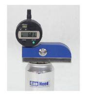
CanNeed-CSG-200 Countersink Gauge (digital) is used to measure the Countersink depth.
